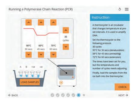
A frame from Learning Science's interactive virtual laboratory on 'Running a Polymerase Chain Reaction'. On this page, users have added all PCR reagents into microfuge tubes and now need to load and set the thermocycler. This is just one of dozens of bioscience interactive resources offered by Learning Science to support students in preparation for their laboratory experience.
